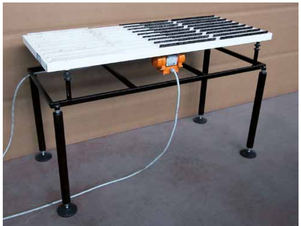
Low friction vibrating table for handling sheet metal
