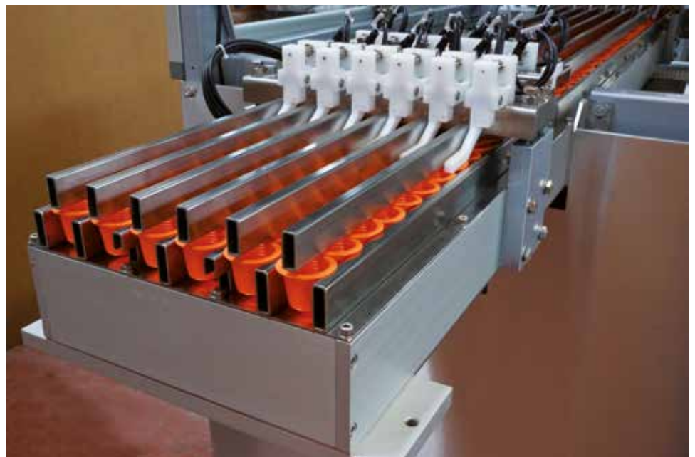
CONV-A 6-row ventilated air conveyor
