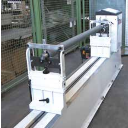
Balancer to check and adjust dynamic imbalance of roller brushes
