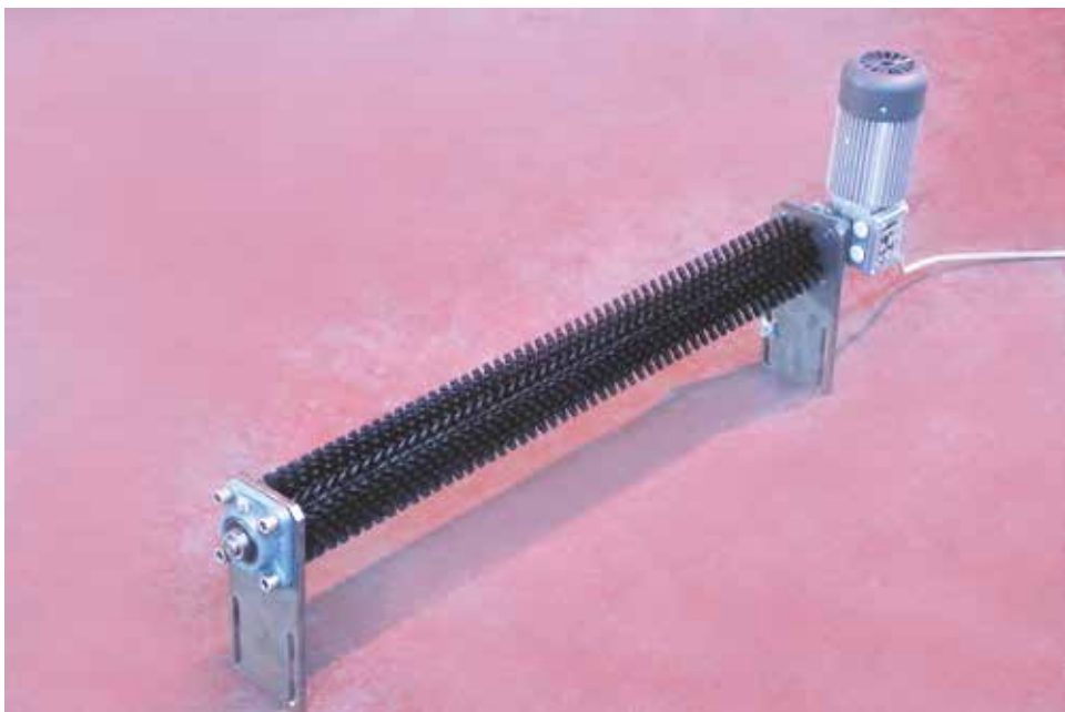
Driven brush for the cleaning of conveyor belts
