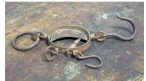
Strain gauge, utilised as a scale for weights of up to 150 kg.
