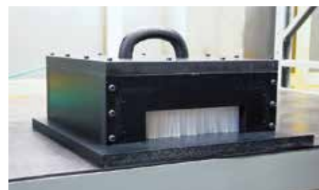
Test rig for acoustic insulation capacity of linear strip brushes
