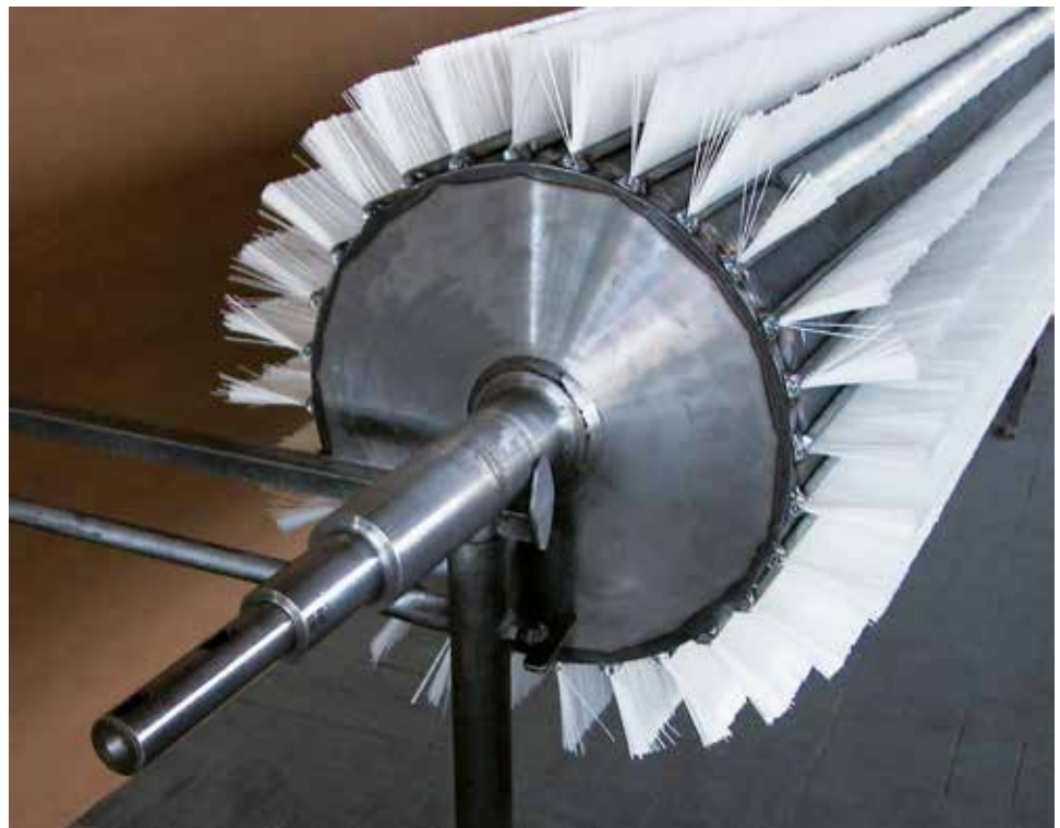
Interchangeable strips on steel core
